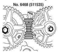
**3.** Follow vehicle service manual procedure to service timing belt as required. Remove tool when finished.
