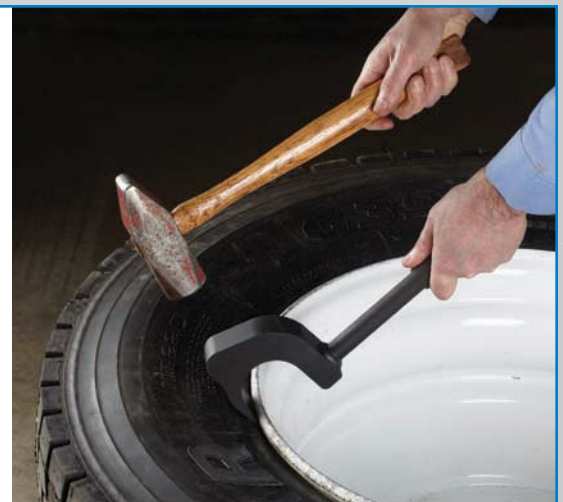
Excellent for damaged tires or tires with weak sidewalls where conventional bead breakers will not work.
