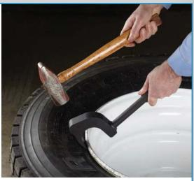
Excellent for damaged tires or tires with weak sidewalls where conventional bead breakers will not work.
