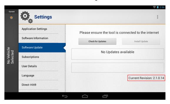
NOTE: User selectable "Check for Updates" and "Install Updates" functions are available as shown. The Automatic background download is always active when connected to the internet.
