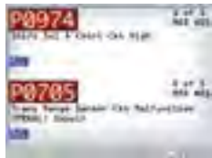
Displays codes and descriptions on the same screen
