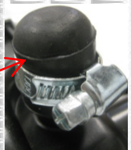
SPECTRA HEATER RETURN LINE WITH RUBBER CAP AND CLAMP (MAY REQUIRE REPLACEMENT EVERY 1-2 YEARS)
