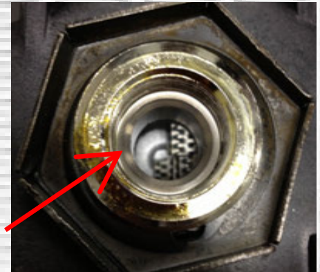
APDI GM STYLE COOLER NUTS WITH OEM DIAMETER OPENINGS
