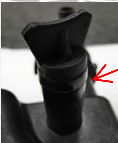
REACH HEATER RETURN LINE WITH RUBBER CAP AND CLAMP
