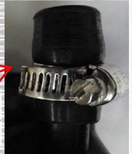
SILLA HEATER RETURN LINE WITH RUBBER CAP AND CLAMP (MAY REQUIRE REPLACEMENT EVERY 1-2 YEARS)
