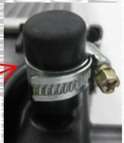
APDI HEATER RETURN LINE WITH RUBBER CAP AND CLAMP (MAY REQUIRE REPLACEMENT EVERY 1-2 YEARS)
