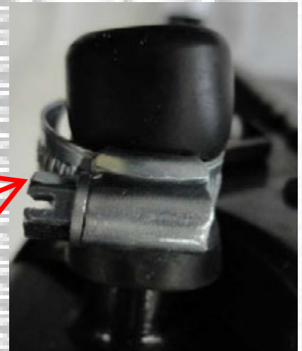
REACH HEATER RETURN LINE WITH RUBBER CAP AND CLAMP
