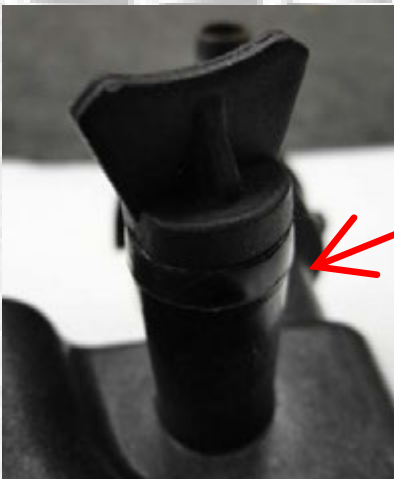
VP HEATER RETURN LINE WITH RUBBER CAP AND CLAMP (MAY REQUIRE REPLACEMENT EVERY 1-2 YEARS)
