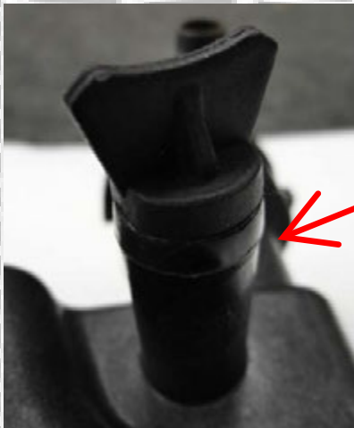
SILLA HEATER RETURN LINE WITH RUBBER CAP AND CLAMP (MAY REQUIRE REPLACEMENT EVERY 1-2 YEARS)
