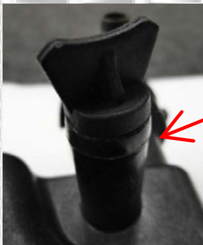
APDI HEATER RETURN LINE WITH RUBBER CAP AND CLAMP (MAY REQUIRE REPLACEMENT EVERY 1-2 YEARS)
