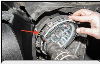
Once the OEM grill is removed, use a T15 torx to remove the headlight adjuster.
