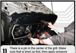
to the bottom of the grill to snap in place.
