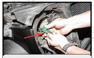
Unplug the OEM headlight adapter from the factory wiring harness.
