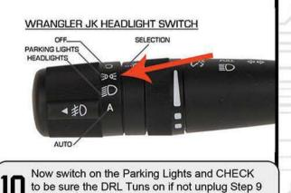
to be sure the DRL Tuns on if not unplug Step 9 and revers the plug direction and test again.
