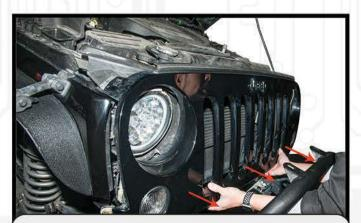
4 Start from the bottom and pull back on the OEM grill to release it from its fasteners.
