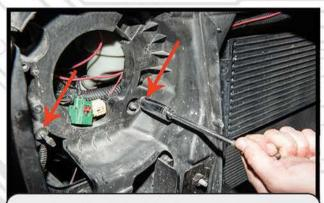
Use a 15mm Socket to remove the two headlight 8 posts. Refer to picture above for the locations.
