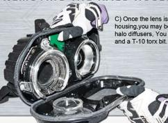
C) Once the lens is separated from the housing, you may begin removing the stock halo diffusers, You will need a 10MM socket
