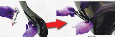
UNCLIP THE STOCK SIDEMARKER, AND THEN REPLACE IT WITH YOUR NEW DRACLE LED SIDEMARKER. PUSH YOUR WHEEL LINER INTO PLACE AND REPLACE YOUR RIVETS.
