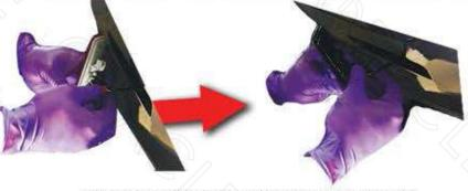
REMOVE THE STOCK SIDEMARKER FROM IT'S PLACEMENT, THEN REPLACE IT WITH YOUR NEW ORACLE LED SIDEMARKER
