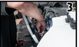
Twist and remove the parking light bulbs, and set grill to the side.
