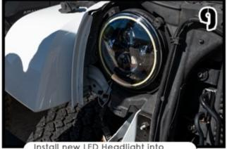
Install new LED Headlight into factory housing on chassis.
