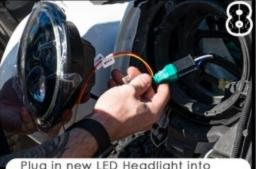
Plug in new LED Headlight into supplied adapters.
