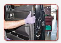
YOU CAN NOW LIFT UP ON THE DOOR PANEL. THERE ARE STILL PARTS ATTACHED TO THE DOOR ITSELF. DO NOT REMOVE THE PANEL COMPLETELY.
