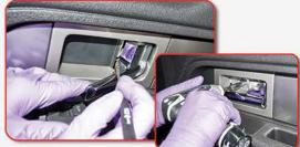
USE A FLATHEAD SCREWDRIVER OR PANEL TOOL TO POP OFF THIS TRIM PIECE. REMOVE THIS 8MM SCREW.
