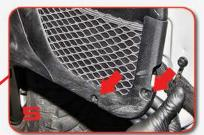
USE A T-20 TORX BIT TO REMOVE (2) BOLTS. BEGIN PRYING DOOR PANEL STARTING FROM BOTTOM. THE REST IS HELD IN WITH CLIPS.
