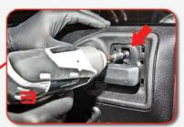
USE A T-20 TORX BIT TO REMOVE (I) BOLT BEHIND DOOR HANDLE.
