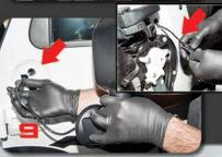
USE A T-35 TORX BIT TO REMOVE THESE TWO (BOLTS) HOLDING THE MIRROR TO THE DOOR.
