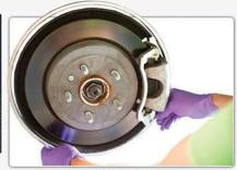
Mock up lighting ring in desired location, generally centered with the brake system. You may test your ring before going any further by wiring it up to any 12 volt power source. Now mark the ring in 3 locations. This is where you will drill into your dust shield and into the ring.
