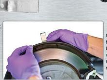
Use the self tapping screws to tap into the dust shield and the bracket at the same time. This will insure that the bracket is mounted tightly to the dust shield.
