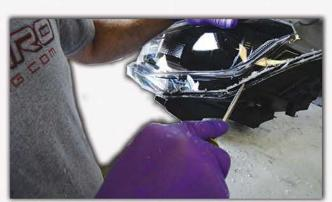
A) Start by using a flat-head screwdriver and apply pressure between the lens and housing. CAUTION! Headlight will be hot.
