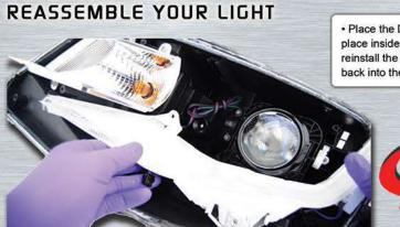
Place the Diffuser back into place inside the headlight & then reinstall the four T-25 screws back into the Diffuser
