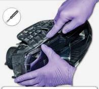
A) Start by using a flat-head screwdriver and apply pressure between the lens and housing. Caution, headlight will be hot.
