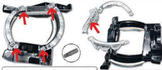
E) Remove the (4) T-15 torx screws. This will allow seperation of the stock halo diffusers.
