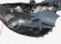
B) Begin seperating the headlight lens and projector bezel from the headlight housing using a Phillips Screwdriver. Pry through the sealant until the two pieces begin to seperate. This step may be difficult, take your time.
