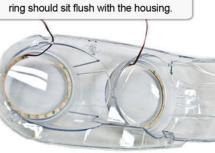
C) Optional: Use additional adhesive to hold the ring in place on the housing.
