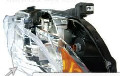
A) Begin by removing the 3M tape backing and fitting the ring to the headlight housing
