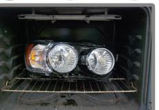
STEP # I: IN ORDER TO OPEN THE LIGHT WE WILL FIRST NEED TO HEAT THE HOUSING. IF USING A HEAT GUN BEGIN BY HEATING THE SEAL EVENTY WHILE CONSTANTLY MOVING THE HEAT GUN. IF USING AN OVEN: PREHEAT TO 225°F AND PLACE THE LIGHT IN THE OVEN FOR IO MINUTES.
