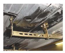
Use bracket #1,2,5 and the cut bracket #4 for the passenger side rear.
