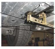
Use bracket #1,2,4,5 and one pc of the cut bracket #4 for the driver side rear.
