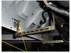
Bracket #4 (cut to length) is mounted to the existing factory holes.
