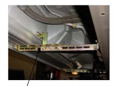
Use bracket #1,2,3 for the remaining installation on driver side only. See above.
