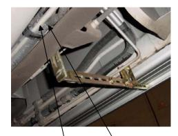
When installing bracket #2 to main frame, check for clearance of AC lines, brake lines etc. behind the main frame before drilling.
