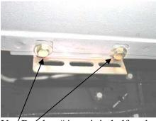
Use Bracket #4 cut it in half and mount it to the factory existing holes on the chassis
