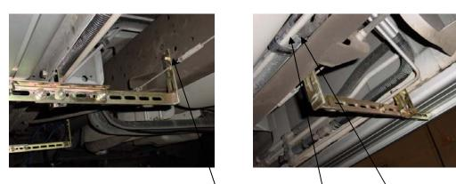
When installing bracket #2 to main frame, check for clearance of AC lines, brake lines etc. behind the main frame before drilling.
