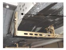
Use bracket #1,2,5 and one pc of the cut bracket #4 for the driver side center. Align and mount the cut bracket #4 to the bottom of the floor to create mounting point.
