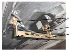
Use bracket #1,2,5 and two pcs of the cut bracket #4 for the driver side front. Start with the driver side front. Cut 2 <sup>1</sup>/<sub>2</sub>" off from the bracket #2 for clearance. Align and mount 2 pieces of the cut bracket #4 to the bottom of the floor to create mounting point. Connect bracket #5 to the bracket #4 mounting point. Loosely attach bracket #2 to bracket #4 and #5. See picture. Repeat procedure on the passenger side front.
