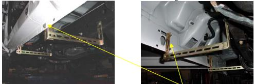
Bracket #4 (cut to length) is mounted to the existing factory holes.
