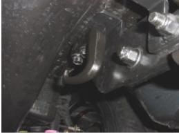
3. Install supplied U-bolt from top of the main frame down thru attached wing bracket holes and fasten with supplied washers and nuts.
