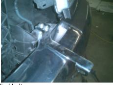
4. Remove factory tow hooks to install brackets with supplied bolts.
