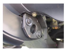
2. With the help of another person, align and position the Brush Guard onto the factory tie down bracket. Securely tighten with the supplied M10X30 hex bolts, washers, and nuts.
