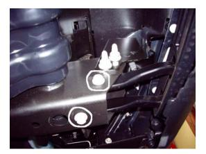
3. Remove the bolts as encircled on the photo above, one under the frame and the other on the inner side of the frame. Place the brackets onto the frame aligning them with the holes from where the bolts were taken out of. Reinsert the bolts and loosely tighten down.
