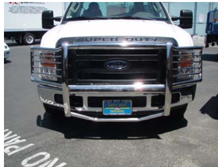
Fully assembled & installed brush guard.
