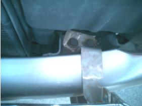
2. Identify main brackets (D for driver side / P for passenger side). Install the main brackets to the main frame by removing and replacing the factory bolts (2 on each side) with the supplied M12x1.75x40mm bolts and washers.
