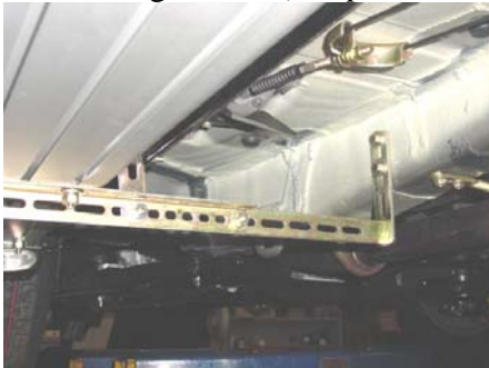
Driver side front using #1,2,5 mounting brackets.
