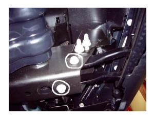
3. Remove the bolts as encircled on the photo above, one under the frame and the other on the inner side of the frame. Place the brackets onto the frame aligning them with the holes from where the bolts were taken out of. Reinsert the bolts and loosely tighten down.
