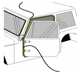
Over time door hinges will wear and cause air to leak between gaps in the door seals. Shimming, realignment, and or possible bending of the top window frame towards the top might be needed for a better seal. If leaks are not corrected wind noise may develop.
