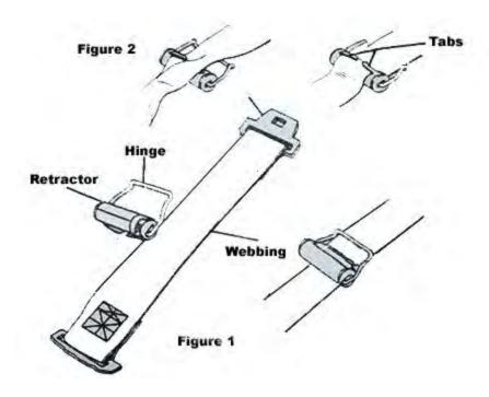
Caution: Do not install retractor to the buckle half of the belt.
