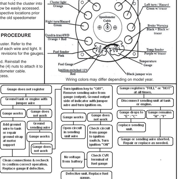
Check all ground points. All ground connections should be cleaned and free of rust and corrosion. If a grounding point has been painted, it must be sanded or cleaned to ensure a proper ground. Please refer to the chart to the right to help track a possible ground fault or malfunctioning gauge.
