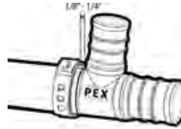
The recommended distance (dimension) between the “Clamp” and “End of the Tube” is 1/8”–1/4”.
