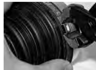
Step 4 Place the clamp over object. Engage interlocking hooks in tightest window position. Firmly crimp the ear with Oetiker pincers.
