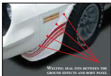
WELTING SEAL FITS BETWEEN THE GROUND EFFECTS AND BODY PANEL.
