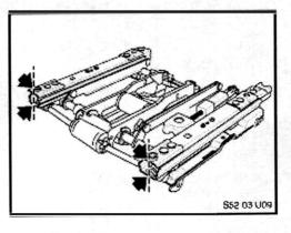
Check the positioning of the upper and lower rails to make sure they are flush. When the procedure is completed on both rails, the alignment of both rails must be identical to prevent binding of the seat when operating. Reinstall the seat.
