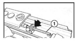
Remove the drive cable (1) from the gearbox and stick it through the guide hole in the rail. Install the screw assembly into the rail and use the drive cable to guide
