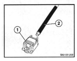
Remove the nut assembly (1) from the adjustment screw (2) and clean off the old grease and dirt from the screw and nut.
