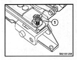
Install the Torx® screw (1) holding the adjustment screw to the upper rail, and tighten to 34 Nm.
