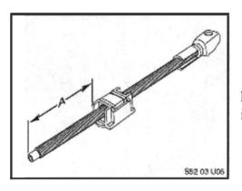
Run the nut onto the screw so that the end of the nut is 90 mm from the cable end of the screw (A).
