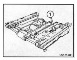
Remove the two Torx® screws (1) holding the anchor nut on the adjustment screw to the lower rail.
