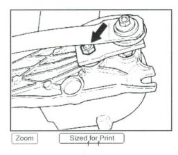
8. Unscrew hexagon nut (arrow) from wiper motor shaft and press off crank arm.
