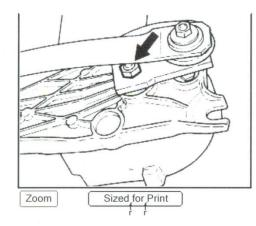
13. Tighten hexagon nut (arrow) to 19 Nm .
