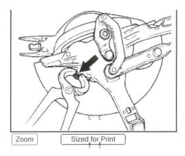
5. On models with air conditioner, additionally attach new rubber seal with a hose strap (arrow).
