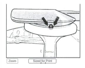
Align markings on gear head for installing (arrows) so that they are above each other (park position).
