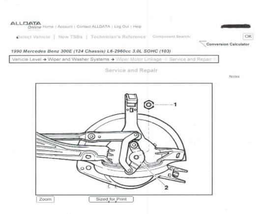
Remove wiper system. See: Wiper Motor\Service and Repair\Remove/Install Wiper Motor
