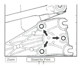
9. Unscrew hexagon bolts (arrows) of wiper motor and take off wiper motor.
