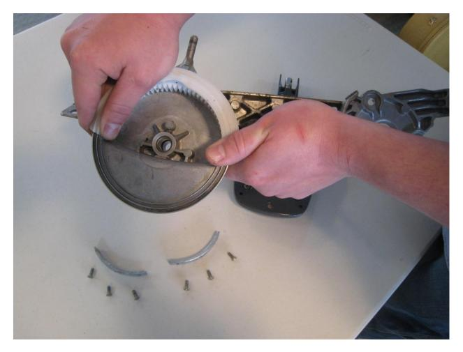
Install the new gear by first getting one side started and then flexing the gear on the other side until it drops into the groove. Install the metal retainers and then the screws. Do not over tighten the screws as the head are easily stripped.
