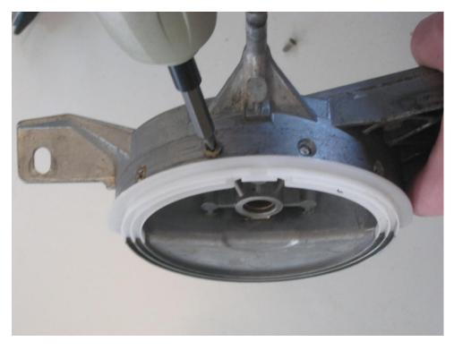
Remove the screws that secure the wiper gear. If you look on the inside you will see the metal retainers that you are removing. Do not loss these are you will be reusing them with the new gear.
