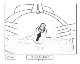
1. Press off locking ring (arrow). **NOTE** : Gear head can only be removed in center position. Do not knock out with hammer. When installing, the push rod must be fully inserted; correct, if neressary, by turning cog wheel (5).
