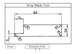
Test Gauge Material: wood or plastic
