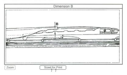
20. Measure reference size "B" with gauge. If the distance is less than 5 mm , bend wiper arm toward windscreen until gauge can be inserted.
