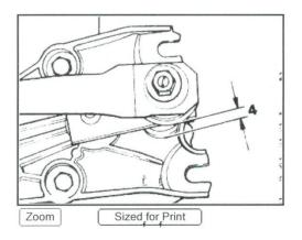
12. Fit crank arm onto wiper motor shaft and align.
