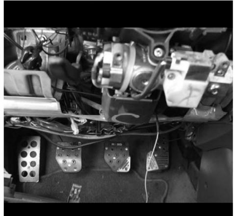
3- Clamp a pin connector to a wire and plug it into the horn wire harness. Run the wire up the steering column.
