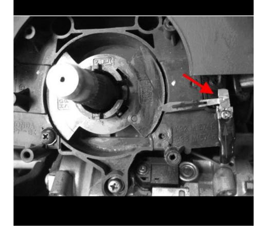
9 - Make sure that the horn contact that was just created contacts the rear of the short hub. The horn connector may need to be bent to accommodate the short hub.
