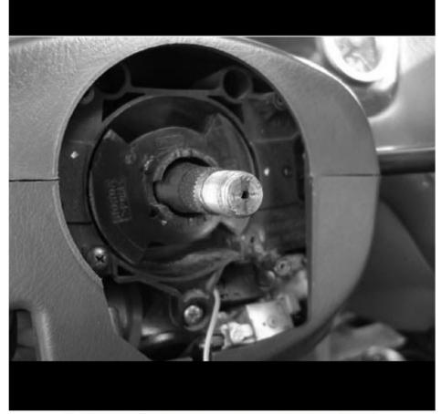
2 - Using a conductivity tester, locate the horn wire on the harness.
