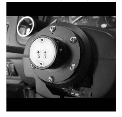
13 - When installing the steering wheel, the components go in this order: Ring garnish (if applicable) <u>Horn button Steering Wheel Quick release base.</u>
