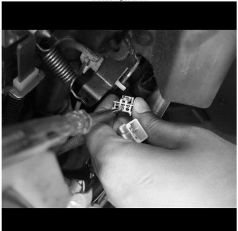
4 - Find something that will conduct electricity that is thin and has good flexibility. We had an old hair clip lying around, and that will serve as our horn contact. (We've also found that other installers have used a variety of things from OEM Shoehorns to cotter pins and conductors.)
