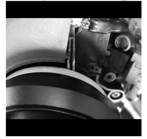
11 - Bolt down the quick release base to the short hub with the supplied screws. Do not forget about the dot signifying the up position. The dot also appears on the base of the quick release.
