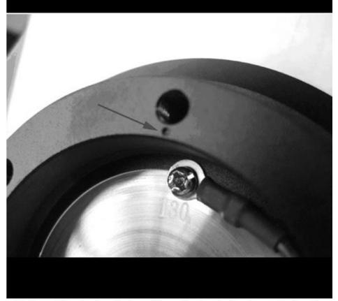
10 - Connect the wires from the base of the quick release to the wires coming from the short hub. The yellow wire will be the hot wire, so connect accordingly.
