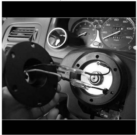
12 – Insert the horn button retainer ring into the top of the quick release body.
