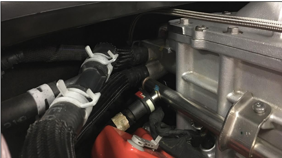
Figure 17 – Reassembled Fuel Rail and Hose Routing
