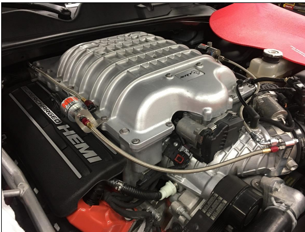
Figure 19 – Assembled Fuel Feed System
