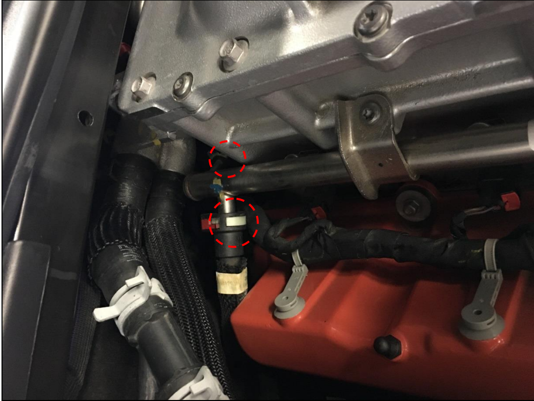
Figure 13 – Fuel line removal
