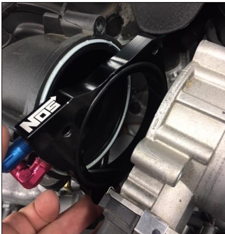
Figure 6 – Nitrous Plate Installation
