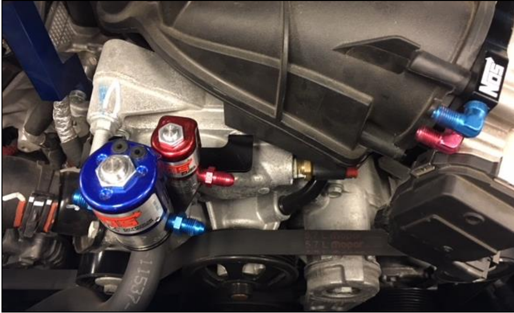
Figure 12 – Solenoid Bracket Mounted Location
