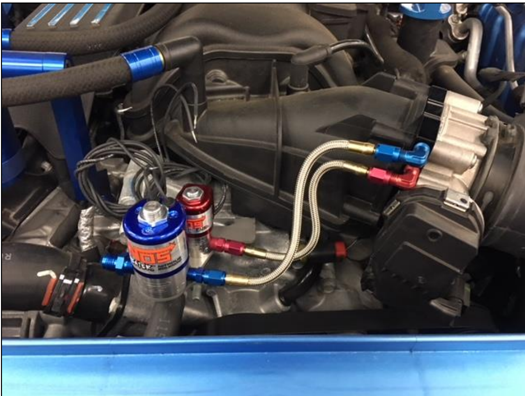
Figure 13 – Installed Nitrous Solenoids
