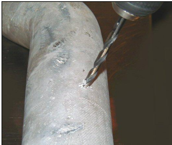
Figure 6 Drill using a 1/4 inch bit.
