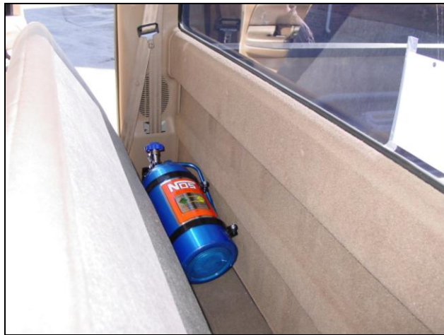
Figure 4 Bottle with blow down tube installed
