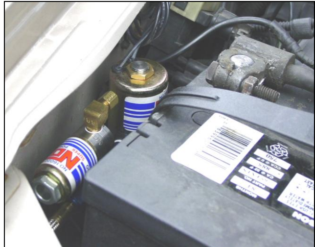
Figure 10 Mounting shown w/ optional purge Figure 11 Completed solenoid mounting
