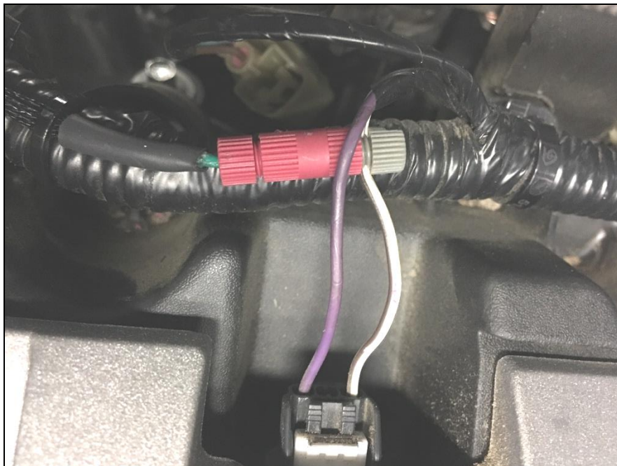
Figure 18 – Tach Signal Wire Connection
