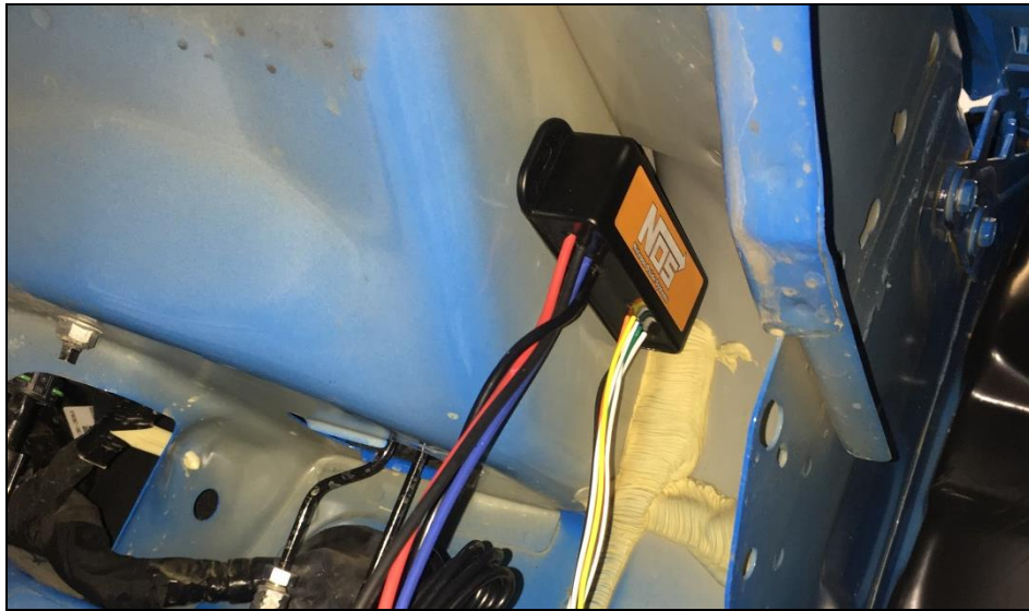
Figure 16 – Mini 2-Stage Mounting Location
