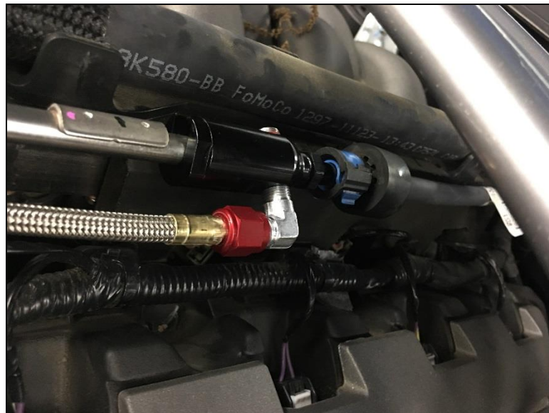
Figure 15 – Fuel Tap Orientation
