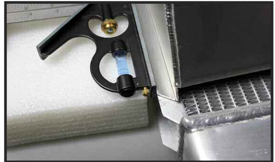
PHOTO 13: Align Radiator & Shroud.
