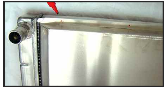
PHOTO 5: Marking outer flanges.
