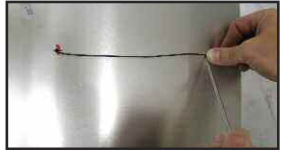
PHOTO 7: Measure and mark circle on fan shroud.
