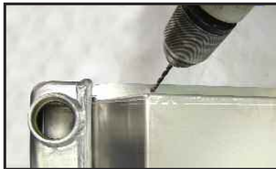
PHOTO 12: Drilling side channel.
