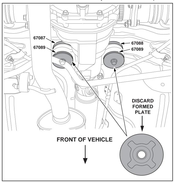
NOTE: REMOVE FORMED PLATE (REFER DIAGRAM) FROM UNDER LARGE WASHERS INDICATED AND DISCARD.
