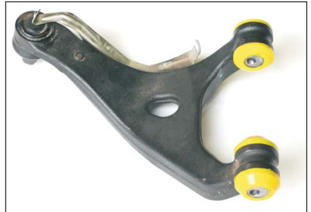
Fig 2 - left control arm with new bushes.
