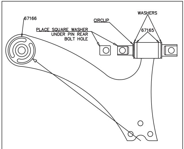
place voiding inline with ball joint as indicated by arrow.
