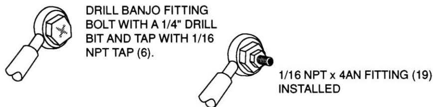
Figure 13 Schematic of “Drilled Out” Banjo Fitting
