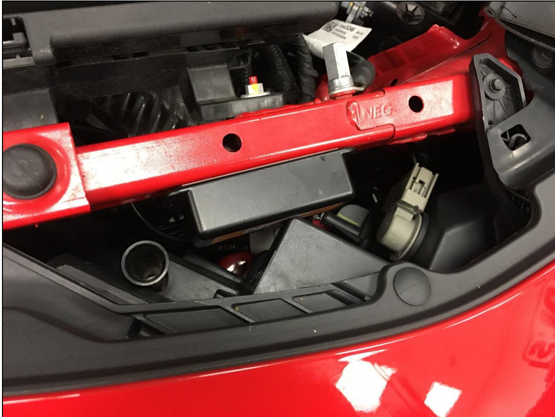
Figure 14 – Mini 2-Stage Mounting Location
