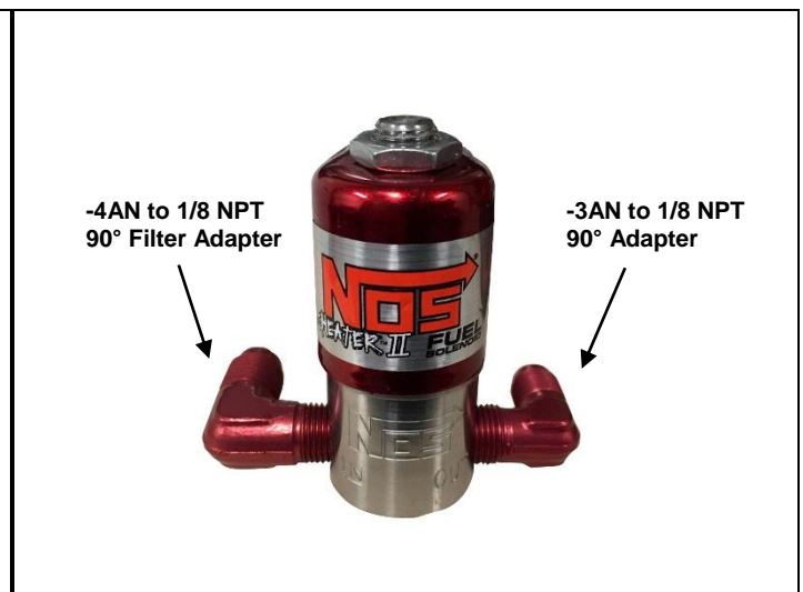
Figure 5 – Fuel Solenoid Adapter Alignment
