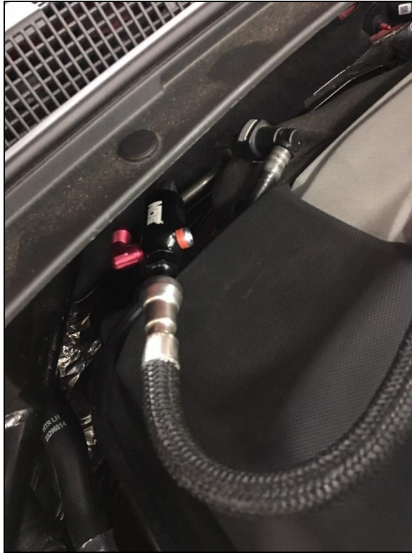
Figure 12 – Fuel Tap Orientation
